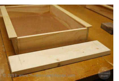
The drawer needs a glide, or lip, on either side of the top so it can slide in and out.
