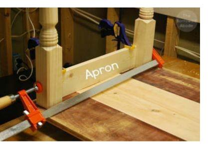
Wedge the side apron temporarily into place between two of the legs.
