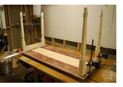
Repeat the apron process on three sides of the desk - both short ends, (the sides) and one long end (the back).
