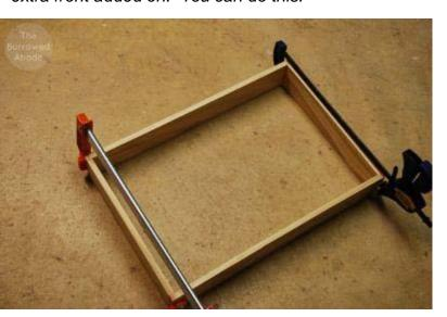
Assemble the drawer sides into a rectangle, using wood glue and small nails.
