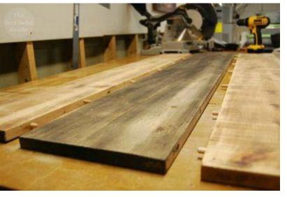
Using the Dowel Hole Jig, drill the holes on the sides of the board.
